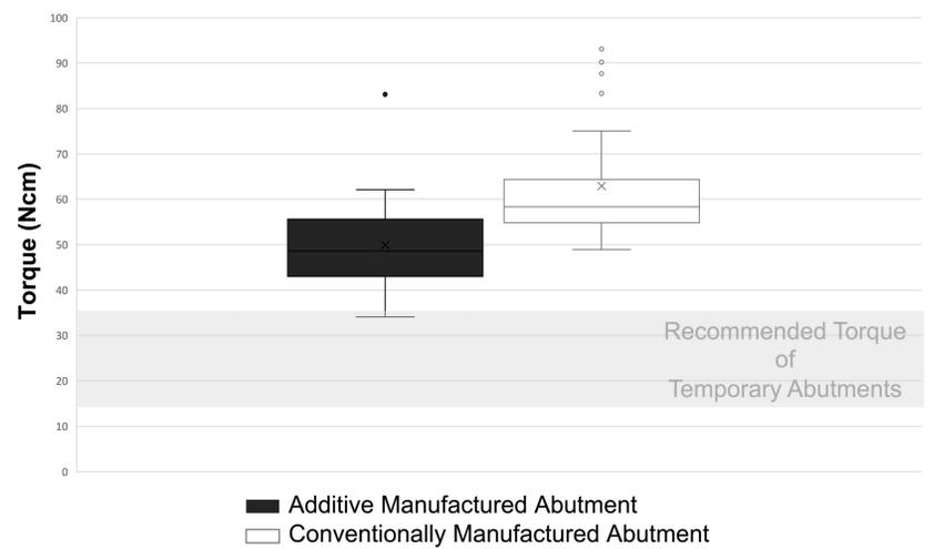
Figure 6. Assessment of torque of novel abutments.
