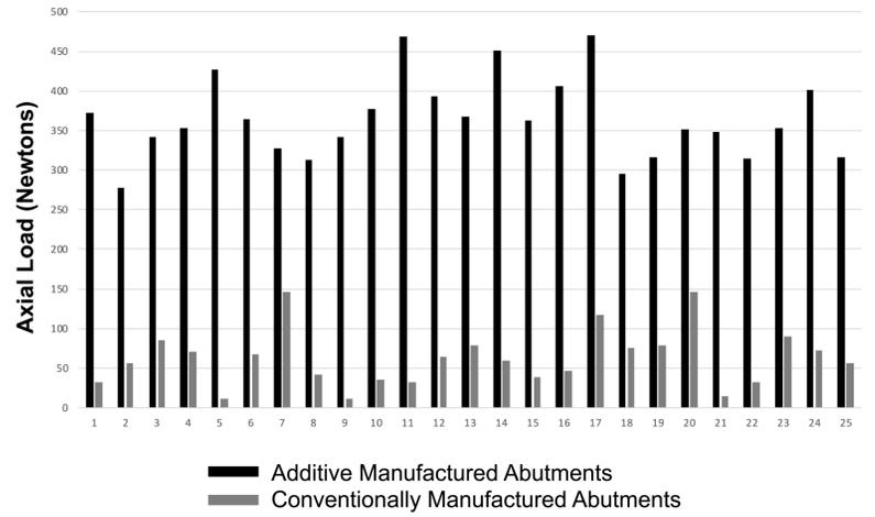
Figure 5. Pin strength of novel abutments.
